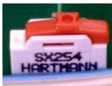
Switch position right (delivery status)
